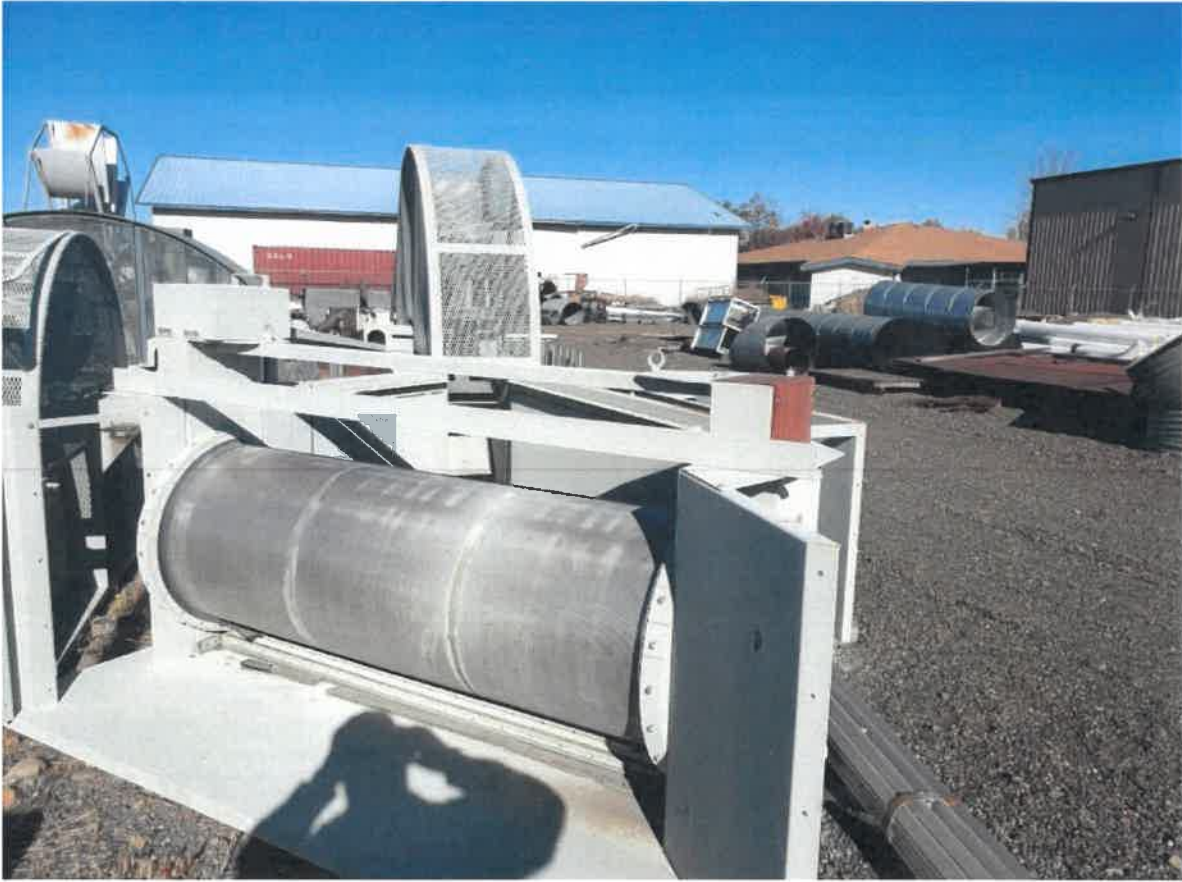
The 24" diameter by 6' length modular drum screen has a max diversion amount of ~3.6 cfs.
